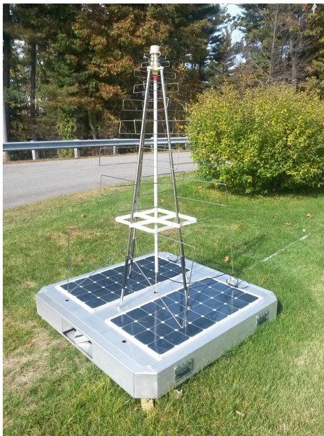
(a) RAPID Field Unit with SKALA antenna.
