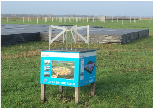
(b) HBA tile (background) and dipole (foreground)
