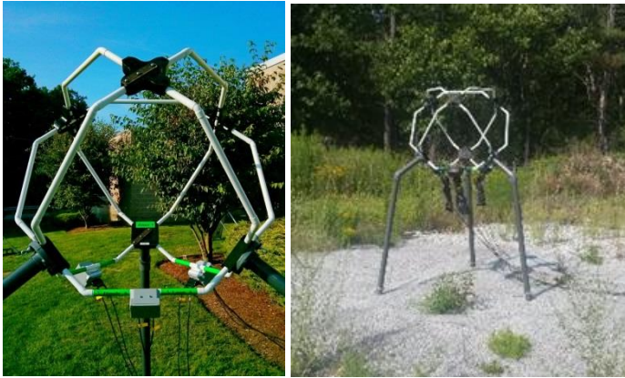
Figure 1. Atom 1 vector antenna at MIT Haystack Observatory. The three octagonal loops that form the vector sensor are white-painted copper tubing and the support posts are PVC. Each loop is 1 m in diameter.
