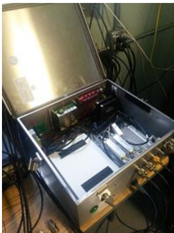
Figure 6. Low EMI receiver box containing Ettus receiver, filters, power supplies, GPS stabilized oscillator, and solid state disks for data recording.
